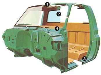
New cab design utilizes larger, one-piece panels whenever possible for better sealing and increased strength.
