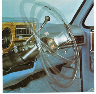
Available Tilt Steering Wheel adjusts to six different positions to suit driver height and seat position. Available with 4-speed manual or automatic transmissions only.
