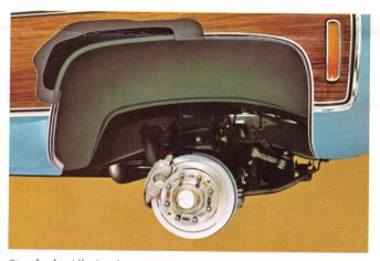
Standard, All Steel, one-piece front wheelhousings protect against spray and flying stones. Because they are undercoated at the factory, they add corrosion resistance while reducing sound levels in the cab. And the single-piston, floating caliper front disc brakes, shown above, are standard on all GMC light duty models. Brake power assist is standard on 2500 and 3500 models; available on 1500 models.
