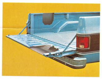
Double-walled Wide-Side Tailgate and Side Panels add strength and warp resistance. The inner panel takes the beating while the outside retains its original good looks. And if you have a camper, you will appreciate that hinges and straps were designed to remove with a minimum of fuss.
