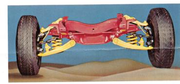
Standard Independent Front Suspension features rubber bushings and rubber control arm dampers on 1500 models for a smooth, quiet ride; 2500 and 3500 models are equipped with steel bushings and rubber control arm dampers for improved ride control. Each wheel is independently sprung to carry the cab over bumps without transferring road shocks to the opposite wheel.
