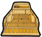
Wide-Side bodies provide high capacity cargo space with double-walled side panels and tailgate. Wood floor available for 8-foot body.
