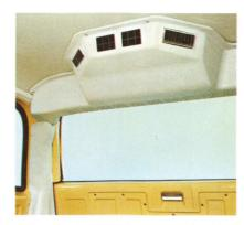
Dual Suburban Air Conditioning adds to driving comfort. Rear unit shown cools and recirculates inside air precooled by front air conditioner. Front air conditioner uses outside or inside air as desired. Ask your GMC dealer for details.
