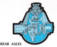
New full floating Salisbury type rear axles are standard on 2500 and 3500 Series models. Quiet running, standard hypoid gearing offers a choice of available ratios for improved performance in most applications. Maximum traction differentials are available in most models.
