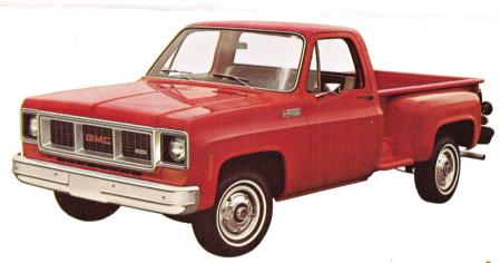
Fenderside models, available in 6½ and 8-foot lengths, feature the convenience of side step loading, smooth interior side walls and an unobstructed floor. Standard pine wood floor contributes to a sure footing for livestock and is supported by strong steel crossmembers. Four-wheel-drive is available for 1500 and 2500 series models.
