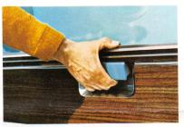
Easy-To-Open Tailgate features one-hand operation with a minimum of effort. The mechanism is enclosed for longer, surer operation. Standard on all Wide-Side models.
