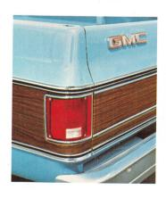
New Lexan® Resin Taillight Lenses are virtually unbreakable. They're made from a material developed for and used on the Moon. Down here, it almost does away with taillight crunch. Wraparound design improves visibility. Standard on all Wide-Side models.
