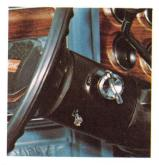
The steering column-mounted ignition switch is new for '73 and incorporates a steering and automatic transmission interlock for additional security.
