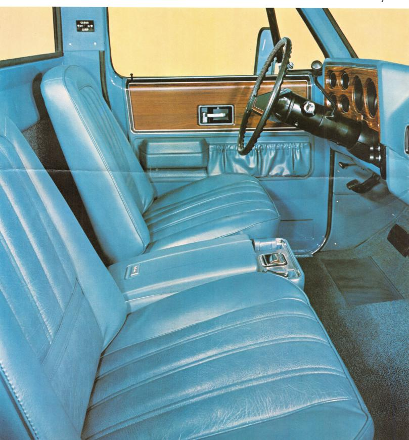
Standard, one-piece integral dash features cockpit styling for the instrument and control area. All controls and gauges are designed for fast driver operation or read-out. Available instruments include ammeter, oil pressure gauge, temperature gauge, as well as clock or tachometer. Resilient control knobs are graphically marked for easy identification. Sierra Grande wood grain vinyl accents shown.
